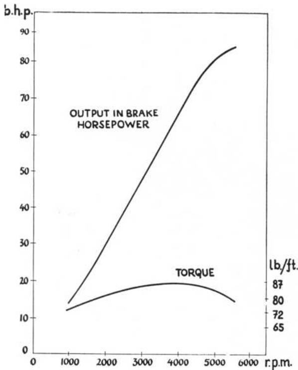
Fig. 3. Output and torque curves.
