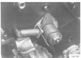
Adjust the camshaft - crankshaft acc. to the markings
