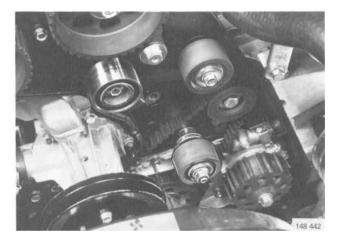
Check the tension and idler pulleys
