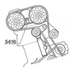
Secure the camshaft gear Use holder 999 5416.
