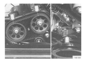
Adjust camshafts - crankshaft according to marking
