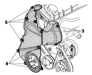
Remove the timing gear housings.
