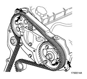
Check that the crankshaft pulley is correctly fitted.
