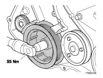
Fit the crankshaft pulley
