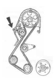
Check camshaft belt tension
