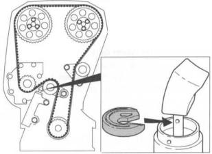
Fit a new plastic washer on the piston.
