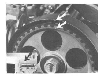
Check that the belt is correctly fitted
