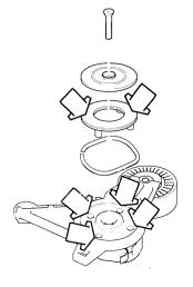
Grease the automatic tensioner pulley (not M/Y 1995)
