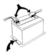
Check that there is sufficient battery acid in all the battery cells. Top up if necessary with distilled water. Check that the battery is properly anchored and connected.
