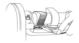
Check the valve clearance for cylinder no. 1 The following values are permitted at inspection:
