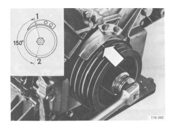
Rotate the crankshaft one revolution to gas exchange cylinder 1
