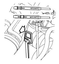
Move the gear lever back and forth between the various gear positions, and keep it in each position for at least 2 or 3 seconds. Select P and wait 2 minutes. Check the oil level.
