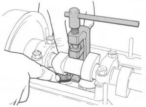
Measure and note the valve clearance for cyl.1
