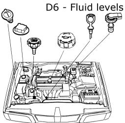
D6 - Fluid levels - engine compartment
