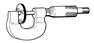
Calculate the thickness of the washer which gives the correct clearance
