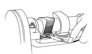
Fit the new washer and remove the tools
