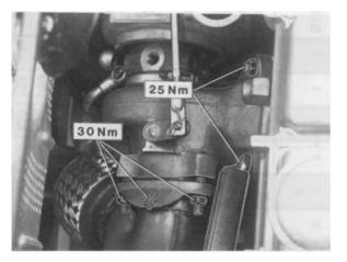
Re-torque of turbo/exhaust manifold
