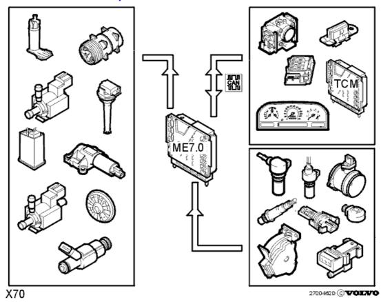
The ME 7.0 (Motronic, Electronic 7.0) is a development of the Motronic 4.4 but also has strong similarities with the DENSO engine management system in terms of the components and their functions.
