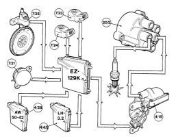
The ICM computes the correct timing of each ignition pulse in response to signals from:
