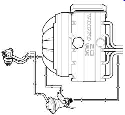
A proportion of the exhaust gases is recirculated to the intake manifold to reduce emissions of nitrogen oxides (NO<sub>x</sub>), which are
