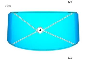
Seal acc. to figure (4) with butyl tape, part number 116 1782, before the rubber strip is reinstalled on the roof panel. Pull out the tape so that it becomes approx. 4 mm thick.
