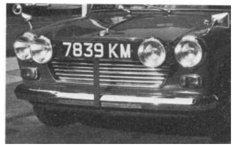
Pat Martin's Morris 1100 has self-levelling lamps in the normal positions, fixed sealed-beams for comparative tests.
