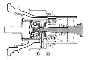
When the EBA unit is activated, the brake pedal/push rod (4) are in principle disconnected from the valve piston (5).
