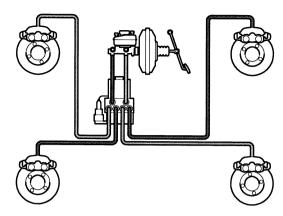
The system has dual circuits and is split diagonally (X-split).
