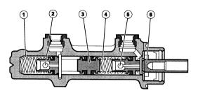
The master cylinder is tandem type, with two pistons - one per circuit. There are check valves in the pistons which close during braking and open when the brakes are released.
