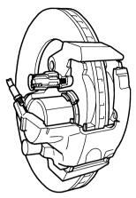
Ventilated brake discs and floating brake callipers with one piston are made of cast iron.
