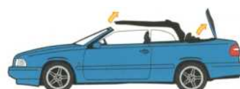
3 The front locks are opened and the top cover is raised.
