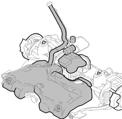
The 850 AWD has a saddle fuel tank with an outer expansion tank. The fuel tank consists of two halves, one on each side of the propeller shaft. Fuel tank capacity is 70 liters.
