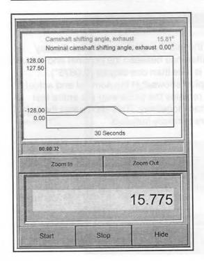
In this screen, the quick test **digital display** shows that the difference between the nominal and actual camshaft setting is more than 15 degrees advanced from what it should be.
