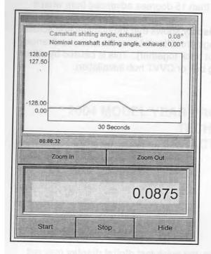
In the screen on the left, the quick test **digital display** shows that the difference between the nominal and actual camshaft setting is less than one degree (0.0875°). The **graphic display** shows that the nominal and actual camshaft setting remains the same over the entire test range (the lines track together). This shows that the belt and CVVT hub are correctly installed.
