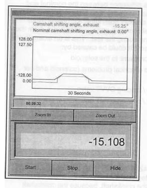
In this screen, the quick test **digital display** shows that the difference between the nominal and actual camshaft setting is more than 15 degrees retarded from what it should be (indicated by the minus sign).
