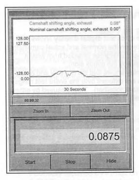
In this screen, the quick test **digital display** may not be helpful to locate the problem. It only shows the instantaneous difference between the nominal and actual camshaft settings.
