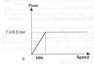
The pump has a constant flow level that feeds an almost constant oil flow to the power steering mechanism.
