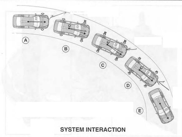
The three systems - AWD, FOUR-C and DSTC - work together in different ways depending on the situation.
