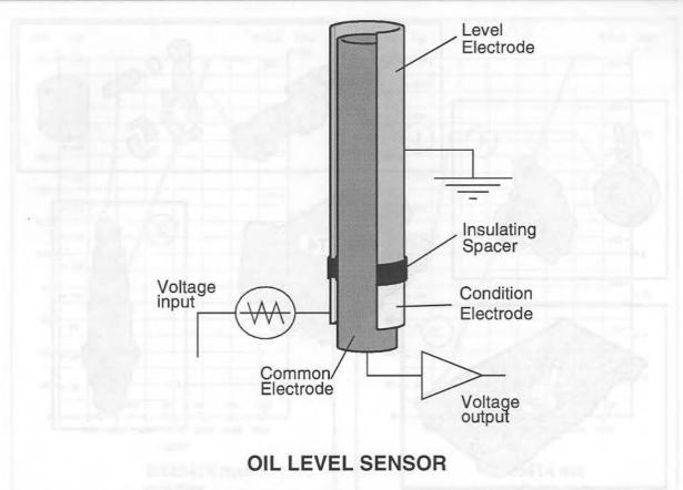
The R engines are fitted with an active engine oil level warning system that tells the driver when the oil level is too low.
