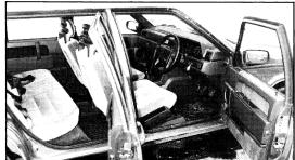
Facia is well laid out, but stereo is an expensive extra. Clear instruments but steering wheel rim masks voltmeter and boost gauge. Sunroof limits headroom for taller drivers, despite front seat's height adjustment
