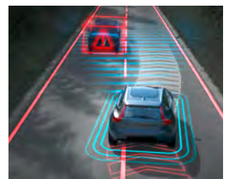
Oncoming Lane Mitigation Using automatic steering assistance, this system helps you avoid collisions with oncoming vehicles. If you drift across the lane markings in the way of an oncoming vehicle, your car can alert you and gently help steer you back into the correct path.
