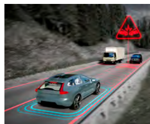
Oncoming Mitigation by Braking A Volvo Cars safety world first, this innovation can detect vehicles heading towards you on the wrong side of the road. If a collision can't be avoided, it can brake your car automatically to help reduce the effect of a collision.
