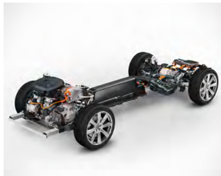
The battery's location helps give your Volvo a low centre of gravity, so it is stable, sure-footed and comfortable while not affecting the car's load space.
