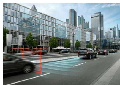
Rear Collision Warning with braking at standstill
