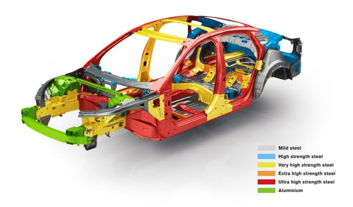
To help keep the occupant space inside intact in a crash, the all-new S90 has literally been made stronger in every sense. This is achieved by more extensive use of hot-formed boron steel, which is the strongest type of steel presently used in the car body industry.
