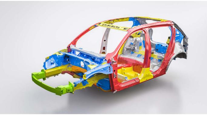
To help keep the occupant space inside intact in a crash, Volvo's new XC40 has been made stronger in every sense. This is achieved by the usage of hot-formed boron steel, which is the strongest type of steel presently used in the car body industry and the construction itself.
