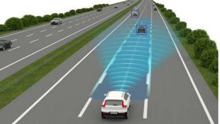
The driver can override the system at any time by using either the brake pedal, accelerator pedal or steering wheel. The turn indicator can be used to temporarily abort the steering support if the driver wants to change lane.
