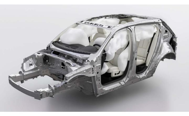
New Volvo cars contain a range of airbags, designed to help protect the occupants in the event of an accident. The collision is detected by advanced sensors that will deploy the airbags when they are needed. The airbags act as supplement to the safety belt and the other protection systems, and are included when needed.
