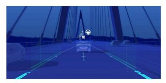
The driver can override the system at any time by using either the brake pedal, accelerator pedal or steering wheel. The turn indicator can be used to temporarily abort the steering support if the driver wants to change lane.
