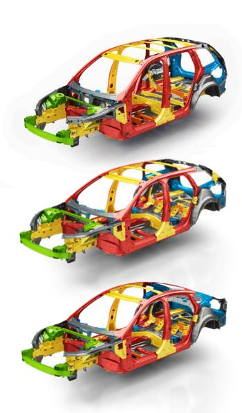
To help keep the occupant space inside intact in a crash, Volvo's new 90 Series cars have been made stronger in every sense. This is achieved by more extensive use of hot-formed boron steel, which is the strongest type of steel presently used in the car body industry.
