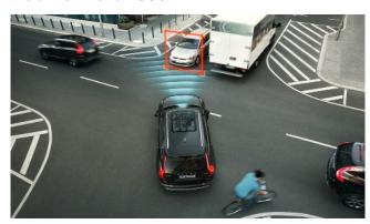
If a collision is imminent, at speeds above 10 km/h, the front safety belts are tightened to secure the driver's and front seat passengers' position.
