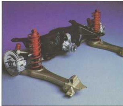
The saloon version of the new 760 has a new split multi-link rear axle for increased comfort and roadholding. The estate version retains the live rear axle which is better suited to carrying heavy loads.
