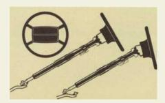
The steering wheel is padded. The steering column has a feature which absorbs shock in the event of front-end collision. It also has a safety breakaway device and a special steering wheel coupling.
