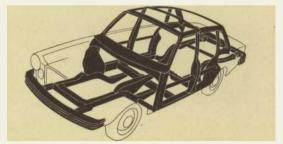
Inside a Volvo, you're surrounded by a steel cage constructed around six boxed steel pillars. Overhead, steel roof supports. Alongside, anti-instrusion bars in the doors. In front and rear, stronger rubberfaced aluminium bumpers.
