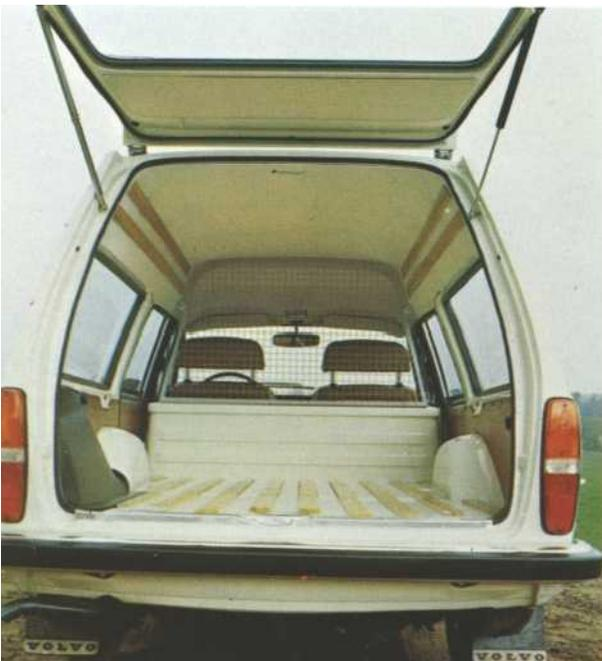
Tough skid rails protect the floor which is about 6' ft. long! This gives almost 85 cu.ft. of space. The width is no less than 56 in. And thanks to the raised roof line the height is practically 40 in. Above the driving compartment where the roof line drops to a lower level the car has a roof rack. Between the cargo area and the front seat area is a very strong steel mesh screen. That's safety for you!
