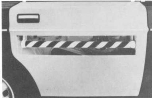
5. Tubular steel side impact barriers in all four door, plus a roll bar in the roof, complete Volvo's all-round protection.
