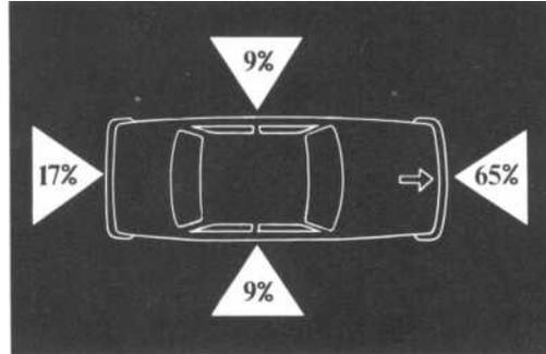
2....,together with actual accident studies, which show front-end collisions to be the most frequent and potentially lethal.
