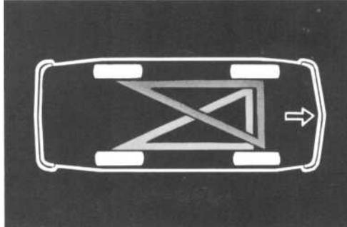
6. Volvo's triangle-split dual brake circuits with new stepped-bore master cylinder. No extra pedal pressure needed if one circuit fails.
