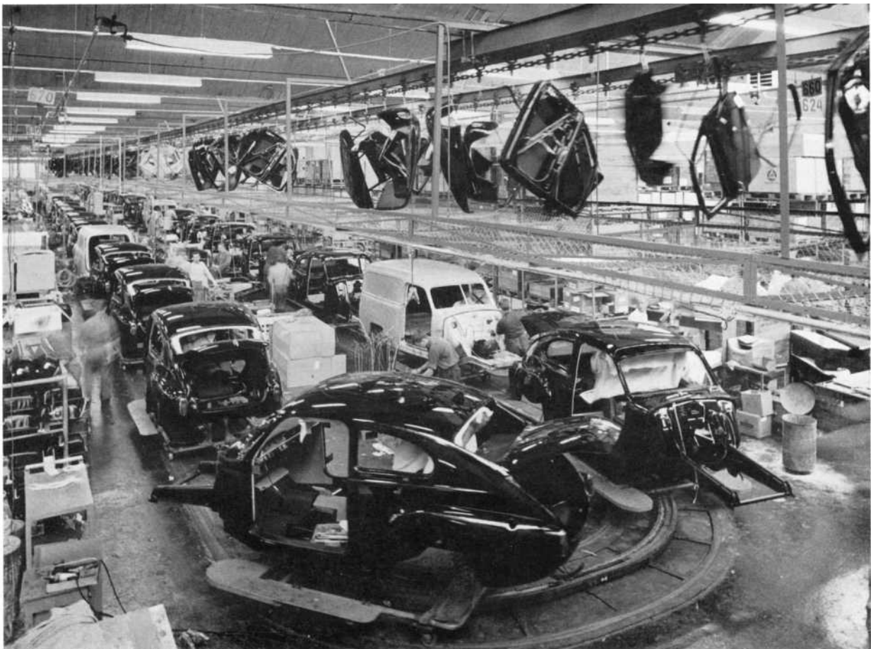
Assembling the Volvo PV 544. The car is ready to drive away one and a half hours from the time that the body from the spraying plant has been lifted onto the assembly line. The main line is supplied with complete sub-assemblies such as front and rear suspension units, balanced wheels, doors and the complete bonnet with front fenders, radiator, grill and headlights from separate feeder lines.
