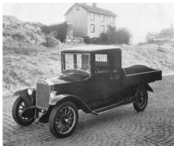
This truck from 1928 had a payload of 800 kg. (1,760 lb.)
