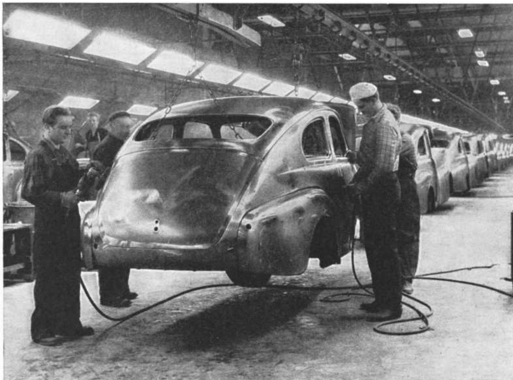
A body being disked before phosphating
