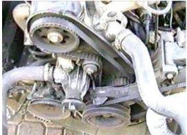
reputable garage). Use a high quality 10mm open ended wrench for the fan bolts. Slack off the power steering pump (loosen top front bolt before loosening the adjusting screw), remove the fan pulley and the top part of the timing gear cover.
