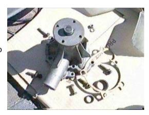
6. The most important thing to remember when installing a water pump, is to clean the block and head (not visible because of angle) surfaces as carefully as possible, before installing the new pump, to remove all traces of the old gasket or
