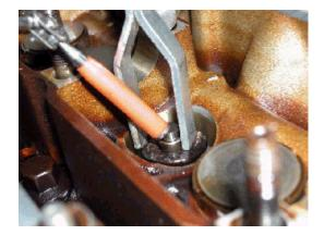
If you haven't done this job before you might want to check the seated depth of the seal be measuring from its top to the end of the valve stem. You want the seals fully installed. I had a machine shop not fully seat the valve guide seals on an engine once. All the seals came up in 50 miles. You never saw so much smoke!
