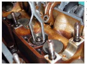
The next picture shows depressiing the valve spring. I am using compressed air to hold the valve shut. Usually you have the bounce the valve compressor a few times to get the keepers to unstick from the valve retainer.
