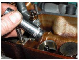
or motor oil to help the seal over the top of the valve. Push the seal carefully over the top of the valve stem.
