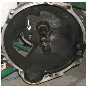
hydraulic clutch. Early Normally Aspirated cars have a mechanical cable clutch; later NA cars have the same hydraulic clutch as turbos. On turbo cars the ball stud for the throwout arm is between the throwout arm opening and the input shaft as pictured to the right.
