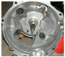
In order to use the NA transmission in the turbo car all you have to do is remove the NA ball stud, and then remove the turbo ball stud and screw it into the NA transmission bell housing. The bell housing has a hex socket cast into it with a threaded nut in it just waiting for you to use. The ball stud from the turbo transmission is internally threaded has a metric stud that screws into it and also fits the nut in the bell housing socket.
