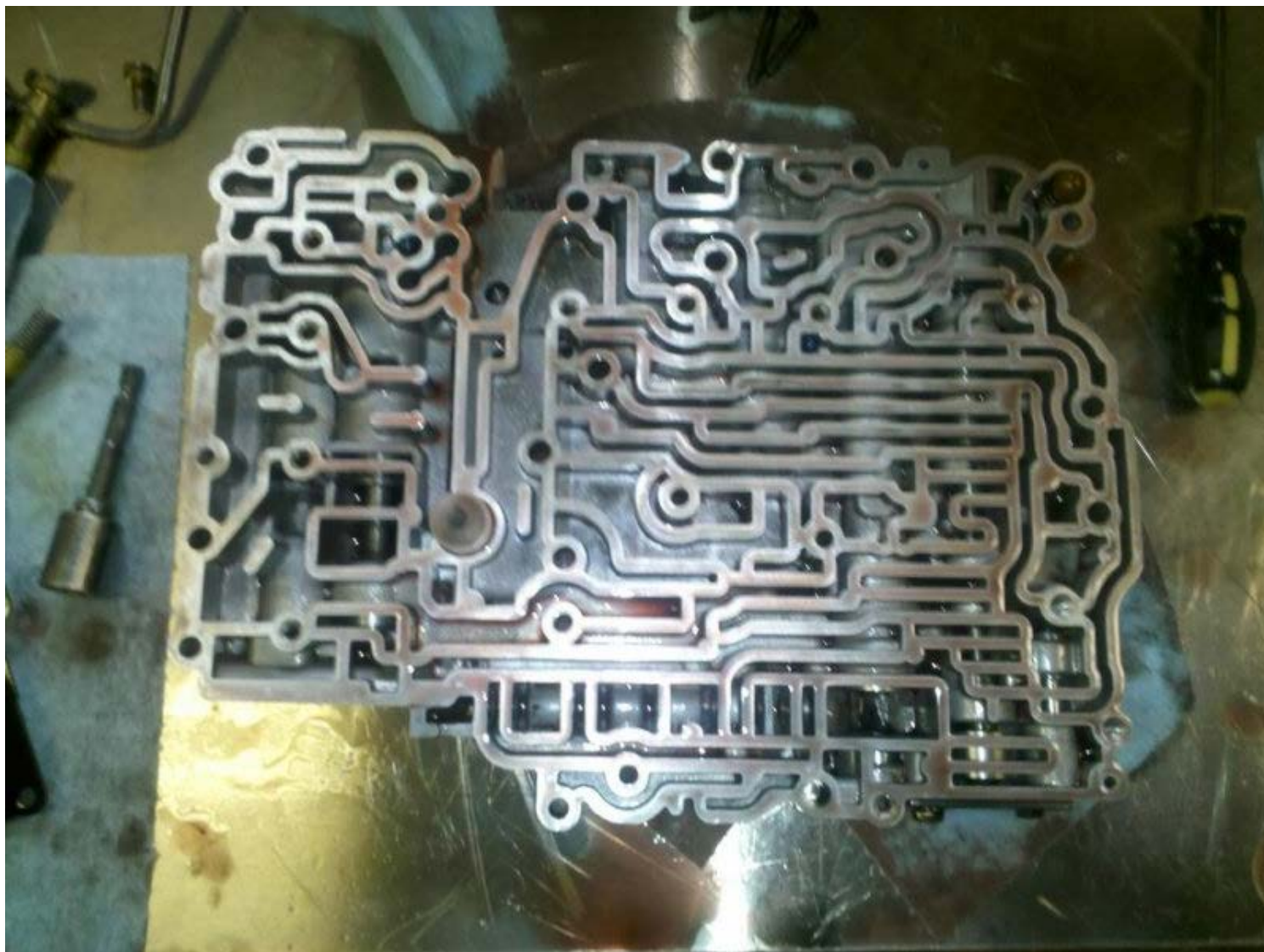
Here's the lower valve body, important locations of things to follow:
