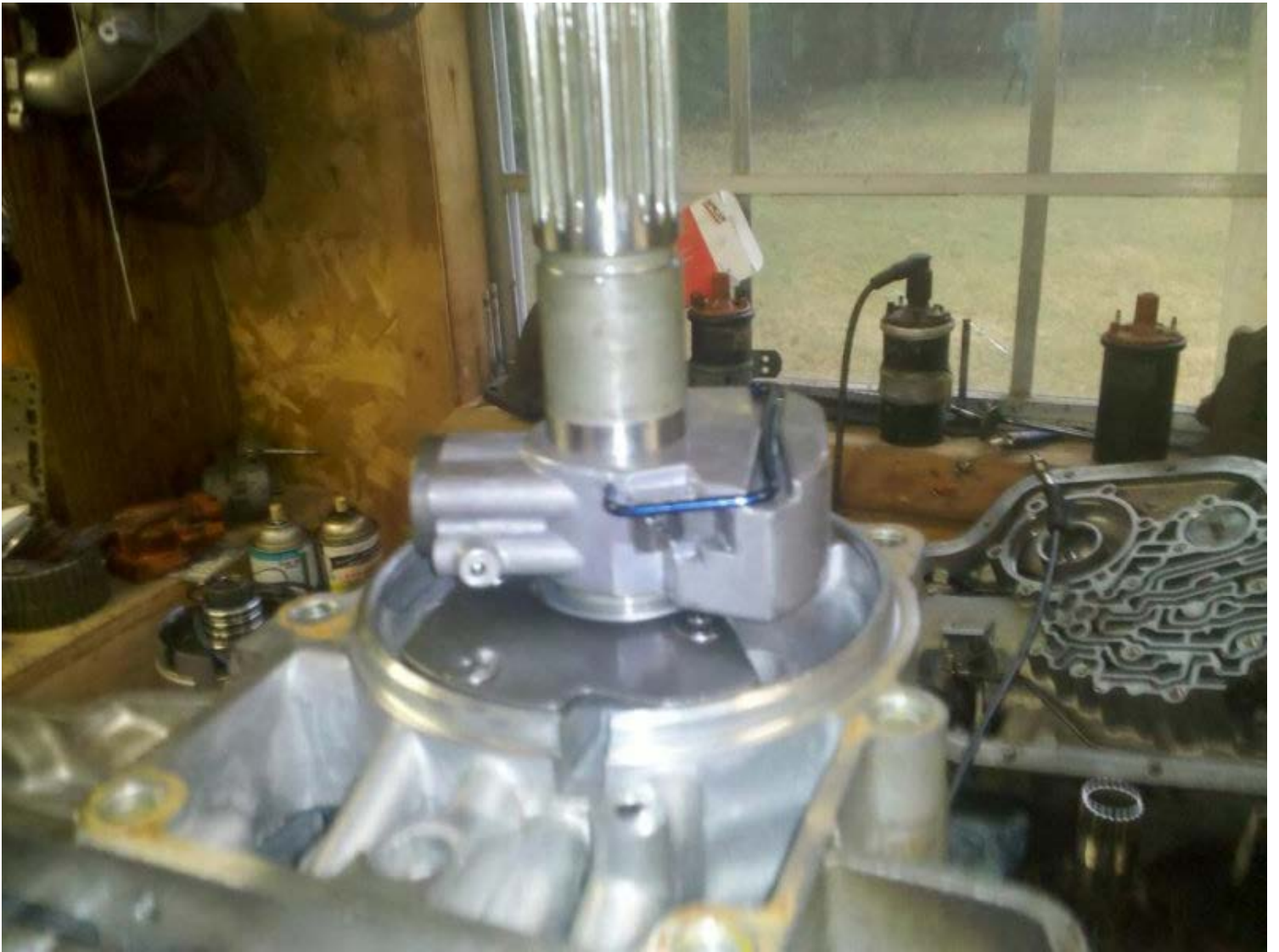
tailshaft housing bolted on
