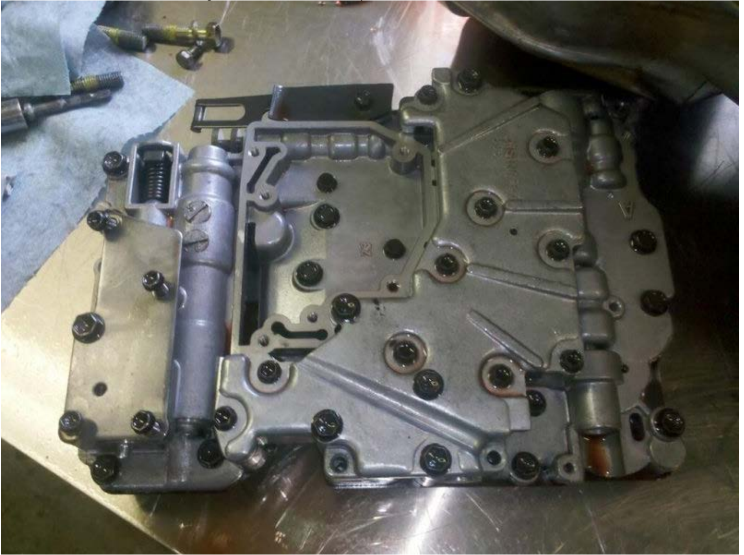
AW71-L (A43DL) valve body, as seen from the pan-side
