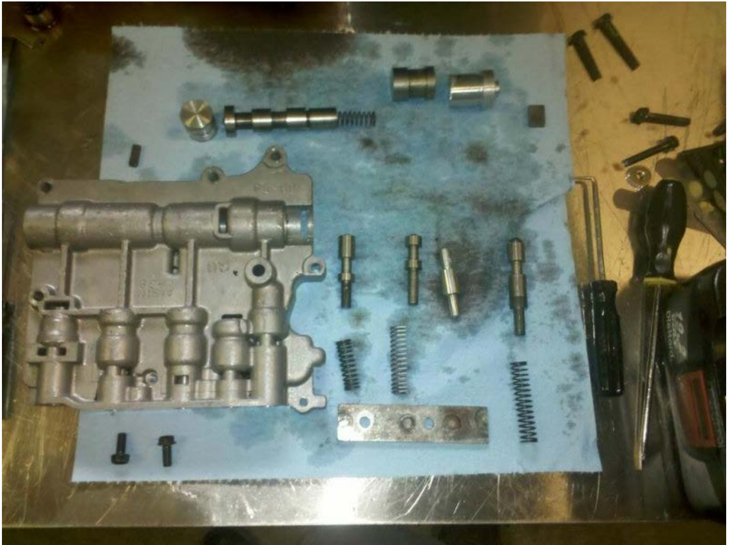
The valve body is positioned correctly as well. There is an additional valve on the end, that didn't fit in the picture with the valve body (orientation remains the same)
