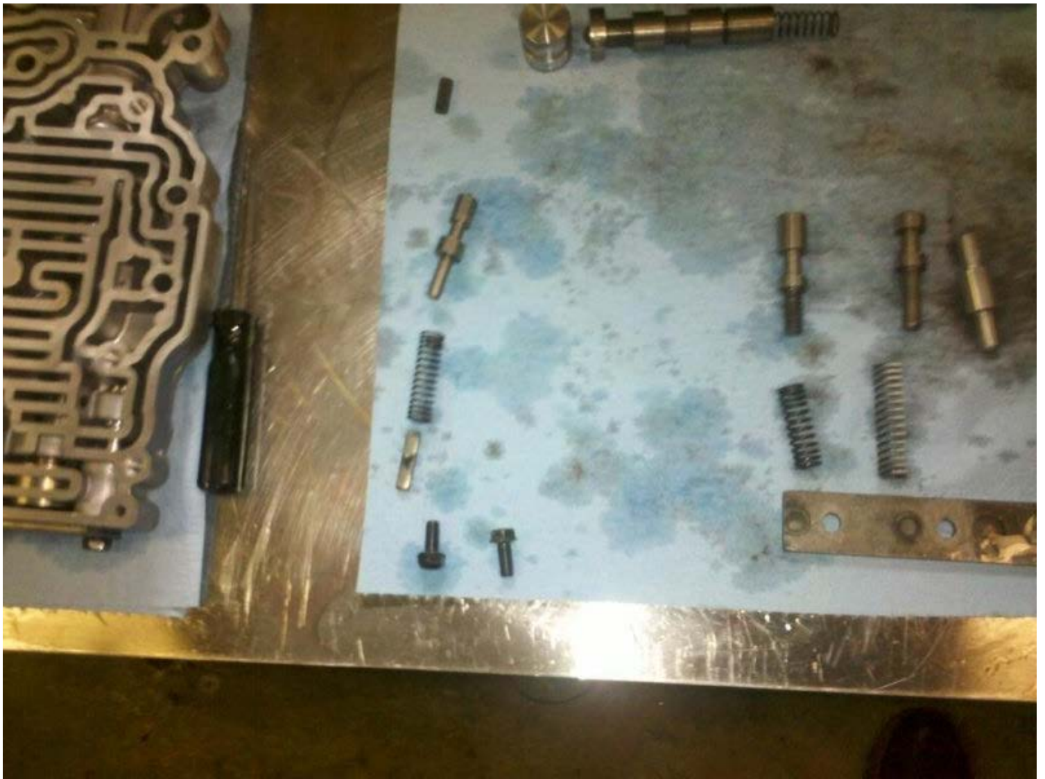
This is the main valve body, disassembled:
