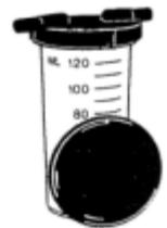
reservoir cap through which you have glued the sampling hose. Run the engine and draw vacuum: gases will rise from the coolant in the reservoir, exit via your hose through the reservoir cap, enter your test chamber by bubbling through the fluid, and if it turns yellow you have an exhaust leak into the coolant.
