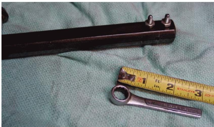
**3. Pan Caps Removal Pin Spanner.** [Randy Starkie] To the right is a pin spanner used to remove the caps under the pan on the Laycock unit. The 3/16" bolts are through a square tube positioned on 5/8" centers with the end of the bolts ground to a radius. This tool eliminates the common practice of using a punch/drift and a hammer to turn the caps.
