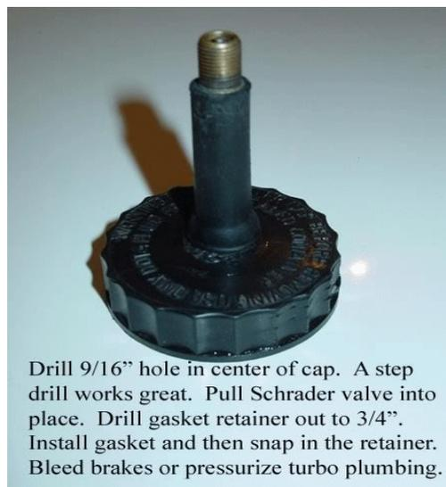
Drill 9/16" hole in center of cap. A step drill works great. Pull Schrader valve into place. Drill gasket retainer out to 3/4". Install gasket and then snap in the retainer. Bleed brakes or pressurize turbo plumbing.
