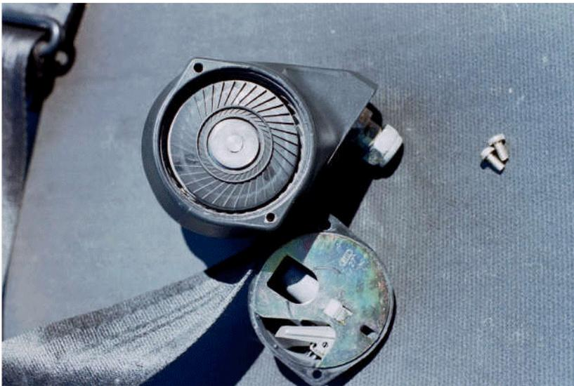
The inertial lock device
