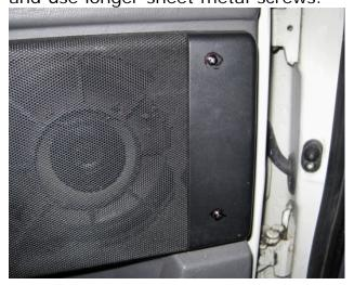
**Speaker Installation**. <u>Crutchfield</u> has an on-line "what fits my car?" application to help you purchase the appropriate sizes. Note that door speakers are shallow and that only those less than two inches deep will fit. Installation is the reverse of <u>removal</u> noted above. Note as well that many 700/900 cars have rear door speaker
