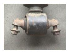
If you fabricate your change to the lower shock mount... a machine shop should be able to do this for minimal cost, or if you have access to the right tools, it shouldn't prove too difficult to fabricate. It's simply a piece of steel tubing that's passed through the lower mount,
