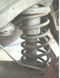
The notes below include two different procedures: wedging the spring out with the trailing arm in place, or unbolting it instead. The latter is much easier. However, unbolting would have been difficult if not impossible had I not had access to the auto shop on base, complete w/ air tools, press, cutoff wheel, grinder, lift, and hydraulic tranny stand. If you have none of these, then you will need to compress the spring and wedge it out.
