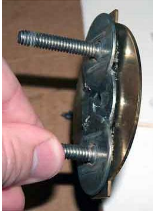
Picture of the mounting bracket glued to the badge. I used J.B. kwik weld for this. I am sure any decent glue will work.
