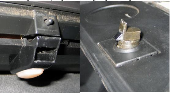
that happens, the door will open. If you own a Dremel Moto-tool, are handy with it, have miniature drill bits (Nos. 60-80), and have some experience taking locks apart and re-assembling, them, you can repair the lock. If not, then you should go to a salvage yard, and remove a lock from a glove box, to which lock the salvage yard
