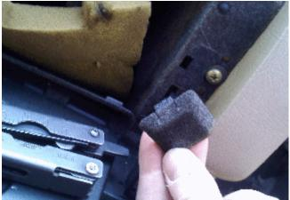
under a black plastic cover, there was a white plastic body fastener which is rotated with the screw slot to remove.
