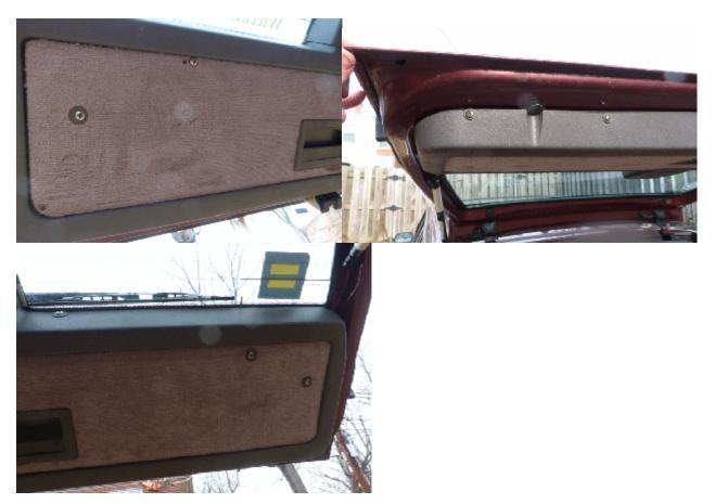
**Removing/Repairing Left Cargo Area Trim Panel.** This is the panel behind which is the gas filler tube. Note that there is not much reason to remove this panel, as the filler cap hinge can be repaired from the outside. This must be why it is so hard to remove. Removal instructions:
