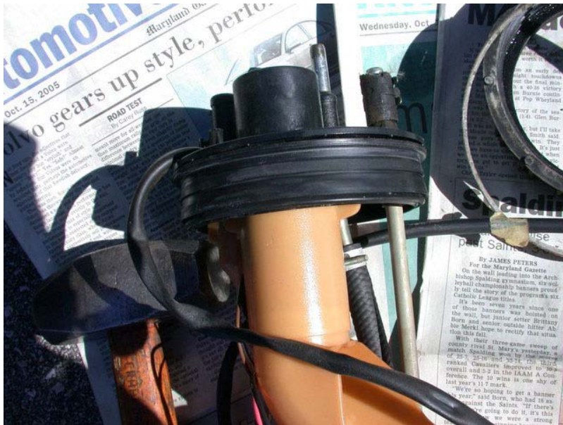
Removing the old pump and comparing it with the new one:
