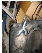
The finished tank repair will be ground down and smoothed after the bulk of the welding is finished. This is a good time to look for porosity in the seams and correct them with another treatment of heat and plastic fill.
