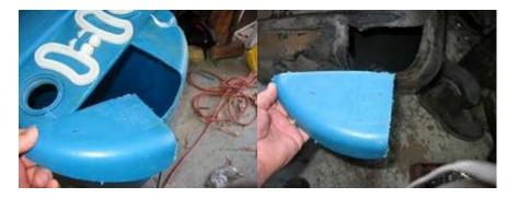
The actual welding is very similar to welding with a torch (brazing) or TIG welding with a fill rod. The hot air is directed at the surface of the plastic in a small circular motion until the plastic starts to look wet. With polypropylene this is around
