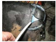
Plastic welding is generally done with either a controlled hot air stream with temperatures around 500 degrees F or with an electric iron device that works in the same manner as a solder gun. Both are fairly expensive at around \$120.00 to over \$200.00 for the commercially available models. Welding rod is also a necessity and can be obtained from most plastics suppliers. For our purpose, this being a polypropylene tank, I am using poly tubing from Home Depot
