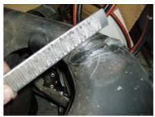
With a little practice the weld is easily worked into beads as the welds on this photo show:
