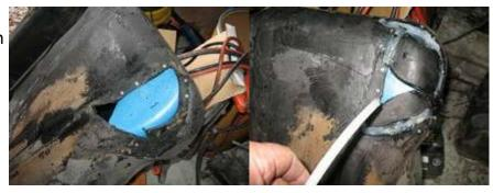
375 to 400 degrees F. The fill material is then fed into the hot air stream and flowed into the area to be welded together. If you are using white poly airline tubing, it will change from opaque to clear just as it melts.
