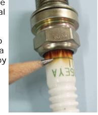
If the spark plug is under-torqued, combustion gases begin to leak past the tapered seat or metal gasket. This leakage causes carbon to form around the threads that, in turn, causes the spark plug to seize to the cylinder head. A properly torqued spark plug will show a bright register mark on the tapered seat or the gasket will show compression.
