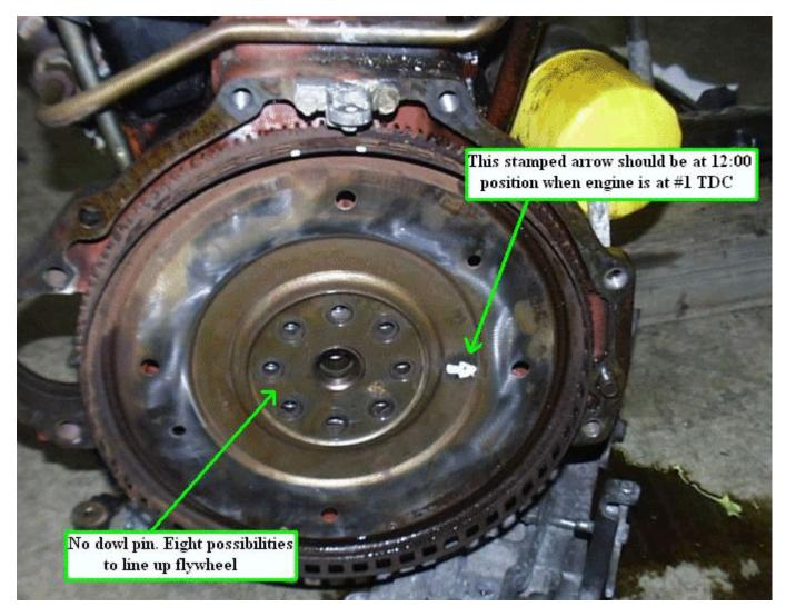
Flywheel Position on Re-installation. [Inquiry:] I didn't mark the position when I removed the flywheel to replace rear main oil seal. How do I replace it?
