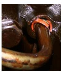
are manufactured with a smaller ridge on them than others. Those tubes would be likely to have the seal slip up and over the ridge. When you reinstall the tube, carefully drive it into place with a mallet, using a wood block as a cushion against the delivery tube. Make sure it fits: some are looser than others. Watch carefully and make sure it is fully seated.
