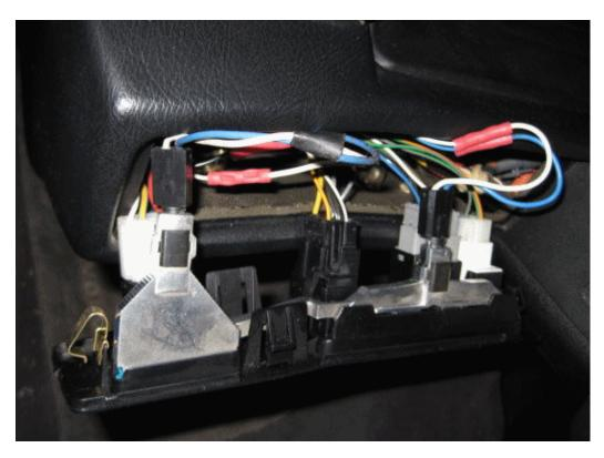
Here is one of the late style in which I've installed an LED with w resistor to trim the voltage. The resistor can't be seen and is down inside the plastic socket.
