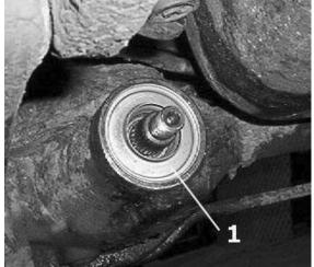
the bearing. Carefully clean the flange where it contacts the seal, removing any rust to ensure the new seal fits. You can use a Dremel with a fine stone to remove rust and clean up any nicks if you are careful. Make sure you install the seal right way around: "outside" is stamped in the metal seal ring. Put a little grease on the
