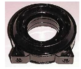
of the center universal joint on the driveshaft. There is a plate that is bolted to the frame rails with 2 bolts per side, the hanger bearing support is bolted to this plate with 2 bolts. The bearing lives in this support. [Editor] Don't drive the car extensively when it has a failing driveshaft support bearing. This can fail catastrophically and send the driveshaft flying at high speeds. When it makes noise, it needs repair very soon.
