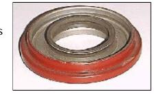
be removed by any reasonable means that doesn't scratch the opening in the diff housing where seal fits. You can put a good-sized screwdriver in between the seal and the pinion shaft and pry it out. It will distort and tear but will come out. Some respondents have not found this very effective: if so, try the following advice to bend the seal housing lip over. Whatever you do, DON'T damage the housing or shaft.
