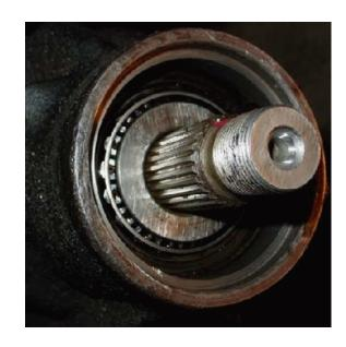
the nut (Volvo recommends a new nut), and tighten the nut to push the flange home. The
