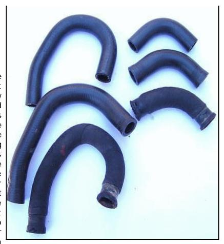
Hose Clamps: For super reliability, use <u>Breeze</u> stainless band Liner clamps which never rust and do not cut your hoses. Volvo OEM clamps are a good second choice; avoid the screw clamps with screw threads cut through them which tend to wear your hoses.
