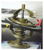
thermostat still leaks after installation, a light coat of RTV between housing surfaces will solve the problem (although it will make cleanup more difficult next time). Finally, you can purchase a new housing for less than \$20.
