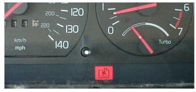
740 and 940 have the indicator position in the instrument panel, but no lamp or sensor (see the photo to the right). Note: Dick Riess contributed a <u>plan</u> for an easier-to-install warning light using a dash switch cutout instead of the panel. See the section at the end below.
