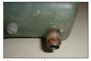
inspect this and not just tighten the hose clamp.[Brian Sullivan] My nine-year-old 945T developed a very small crack in the top of the reservoir... it bubbled a bit when the engine was hot. When I pulled the outlet hose off the bottom of the old tank, the bottom 1/4" or so of the plastic crumbled and fell in the hose. Also, one of the interior plastic walls had broken, and a chunk was floating in the tank. [Editor] These tanks will embrittle over time and should be changed as a "wear"
