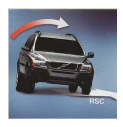
The car's angle and the roll-over risk are both registered by an electronic sensor. At a predetermined risk level, the RSC (Roll Stability Control) system is immediately activated, helping you to maintain control.
