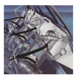
If you nonetheless end up in a situation in which the car rolls over, the inflatable curtain is deployed to help protect the heads of all the occupants and keep all within the car. At the same time, the safety belt pre-tensioners are activated in all the seats, keeping you firmly in the seat.
