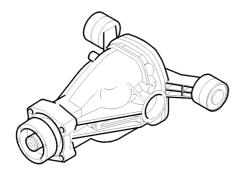
housing and rear cover. The 1165 final drive always has an automatic differential lock.
