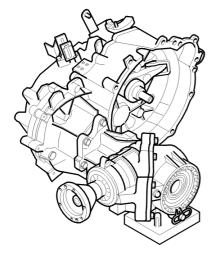
To provide the car with four-wheel drive, transmission M56 has been modified (and given the designation M58) so that power can be taken off to a bevel gear.
