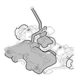
The 850 AWD has a saddle fuel tank with an outer expansion tank. The fuel tank consists of two halves, one on each side of the propeller shaft. Fuel tank capacity is 70 liters.
