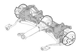
This version of the 850 has multi-link rear suspension. It is the same type as on the 1995 model year 960 but has coil rather than leaf springs.
