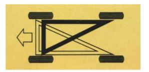
Volvo's triangle-split brake system. Each circuit brakes simultaneously on both front wheels and one of each of the rear wheels. You could lose half your brake system and still keep abt. 80% braking power.
