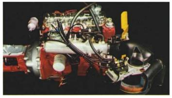
There are four engines in the Volvo power programme. For the 140-series we offer: B 20A 90 hp SAE single carburettor.
