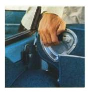
It's an easy matter to fold down the rear seat backrest and arrange a flat cargo area which is 74"/188 cm long. The backrest is dropped, from either side. The seat fixing mechanism has been improved for easier action and it now moves into place in one smooth movement.
