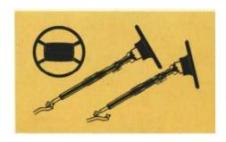
Two-part steering rod with collapsible upper sections in the rod and column. The padded hub of the wheel aligns with the driver's body under impact.
